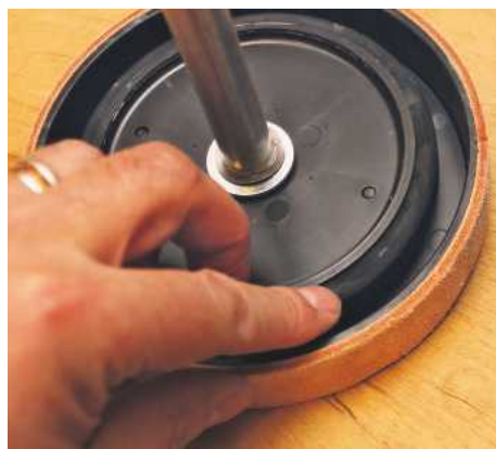
▲ The roughened pin drives both wheels and rests against a rubber wheel for grip to drive
